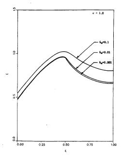
Fig. 2 Fluid-phase skin-friction coefficient vs position.
