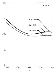
Fig. 1 Fluid-phase displacement thickness vs position.
